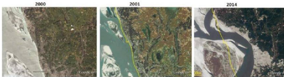
Figure 48 River bank erosion along the Jamuna River near Guthail (Satellite imagery)
